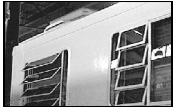
Torque windows allow for good venting in all kinds of weather.
