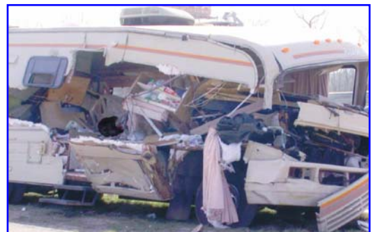
The motor home involved in this collision had a solid wall.
