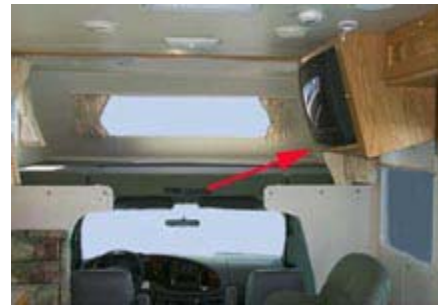
TVs in this class C were recalled because they were found to be loose in the cabinet. (illustration 2)
